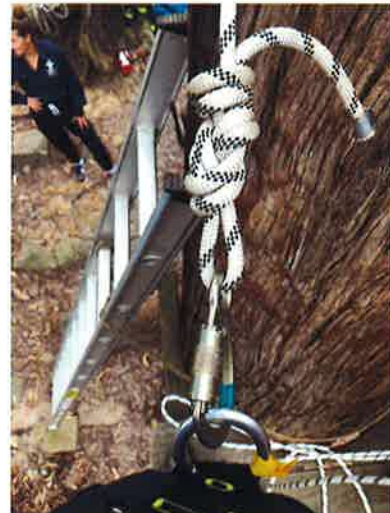
Figure 1.2: Rethreaded figure 8, with stopper, attached through front 'D' on Harness.
